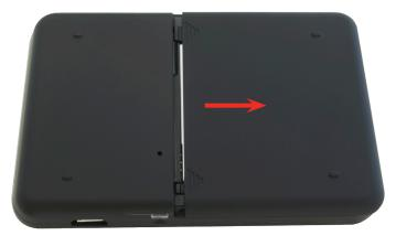
2 Insert the battery by lining up the gold contact points on the battery with the gold contact points in the battery compartment.
