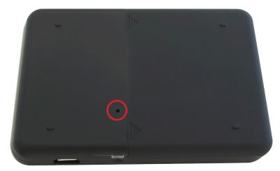
Insert a paperclip into the hole and hold the button down for 5 seconds until the Power LED goes off.
