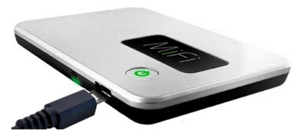
**6** Plug the other end of the AC wall charger into the appropriate electrical outlet. Charge for at least two and a half hours.
