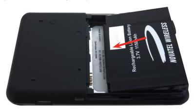
3 Once the battery is secure, place the battery cover back on the device until it locks into place.
