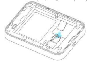
5. Remove the SIM card by gently pressing down and sliding outwards.
