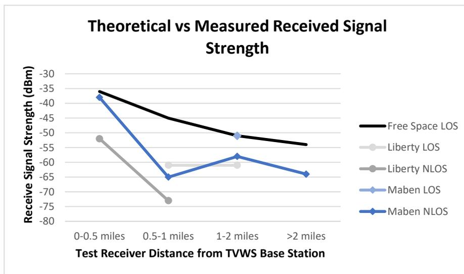
**Figure 1: Theoretical and Measured Received TVWS Signal Levels Averaged at Various Distances**
