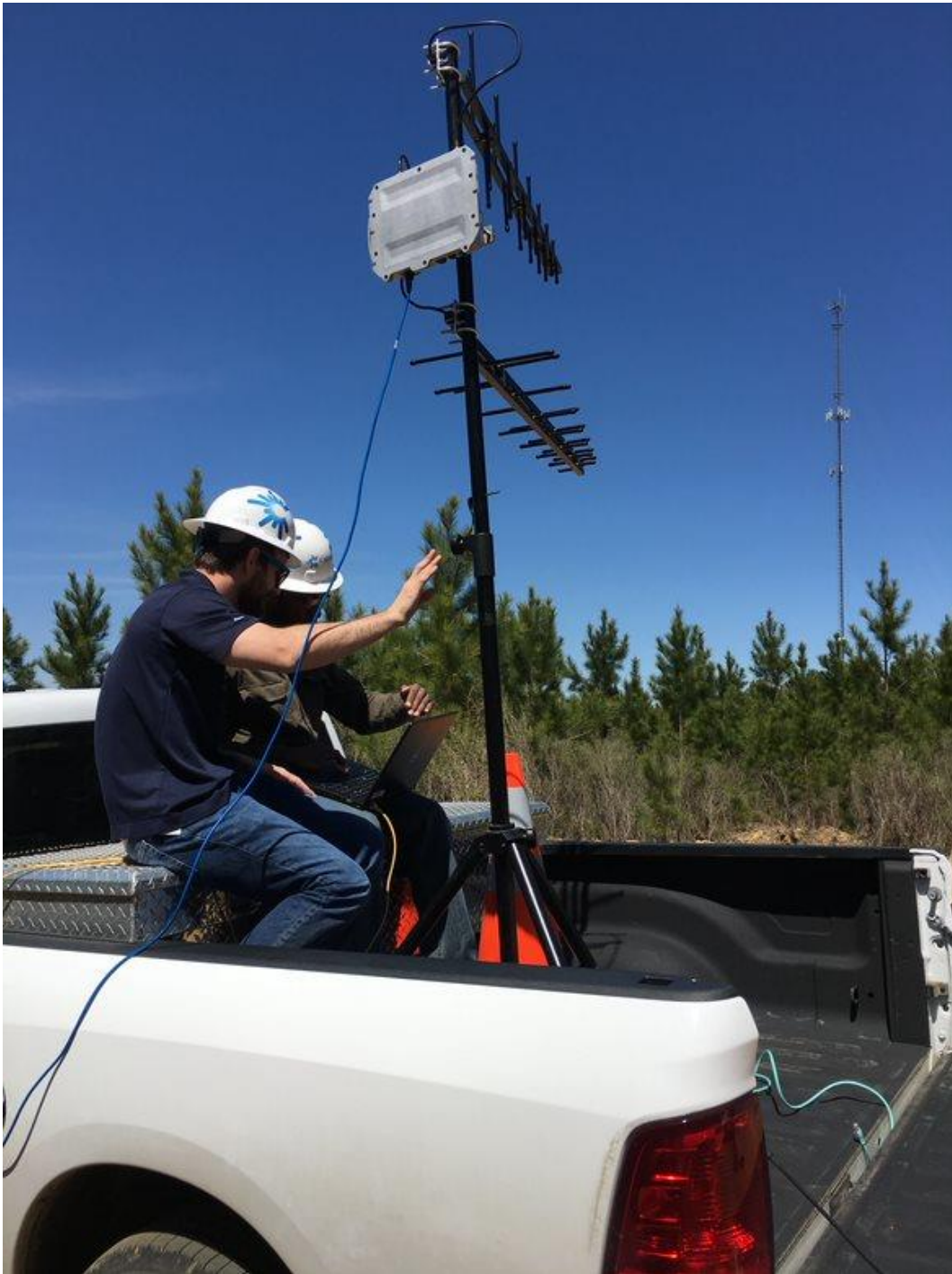
Figure 3: C Spire employees configure TVWS receiver for testing; Maben tower with TVWS base station in background
